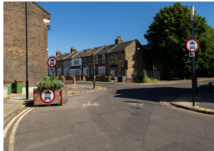
Keogh Road modal filter, implemented as part of Atherton LTN during experimental stage
