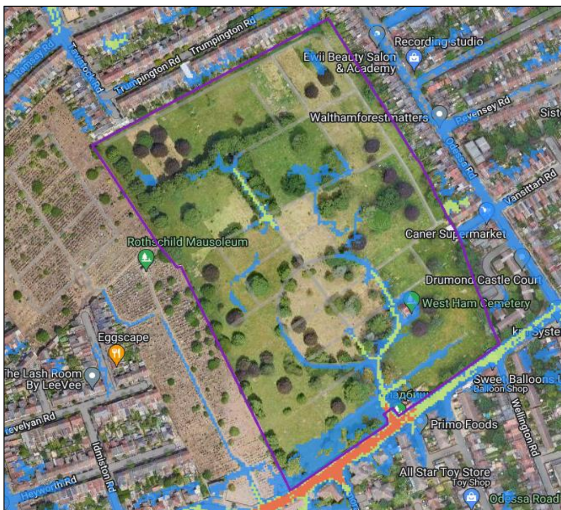
Figure 32: Land subject to 1:1000 year surface water flooding at West Ham Cemetery (Source: Environment Agency, 2024)
