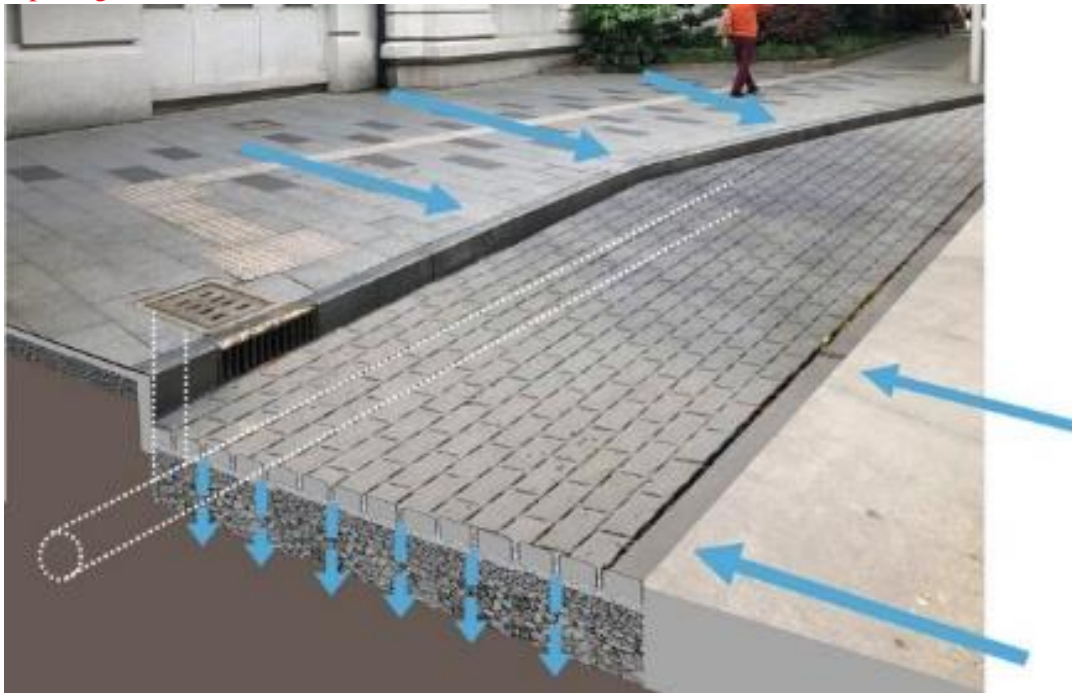
Figure 78: Example of permeable paving (Source: Arup).
