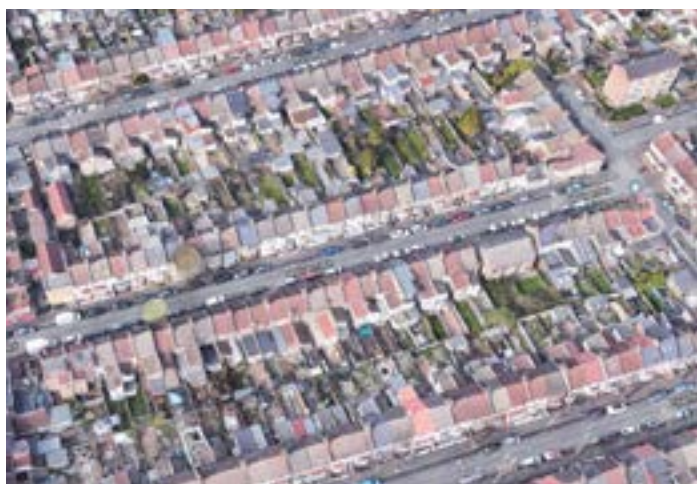
Typical historic residential street layout with row houses face the street in a perimeter block with private gardens in the centre of the block.
