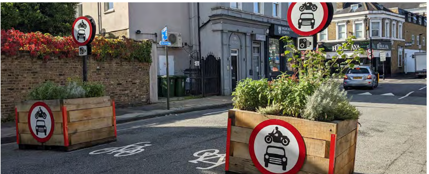
A temporary modal filter in an experimental Low Traffic Neighbourhood in Newham
