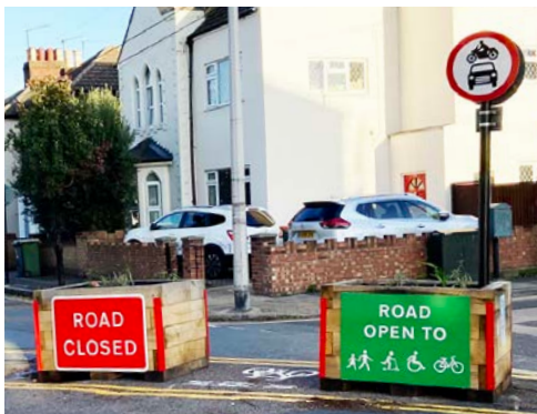
Example of access restriction for motorised vehicles
