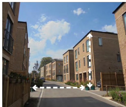
Figure 2.9b: A new suburban street where separation between front elevations is equal to the height of the elevations facing the street.
