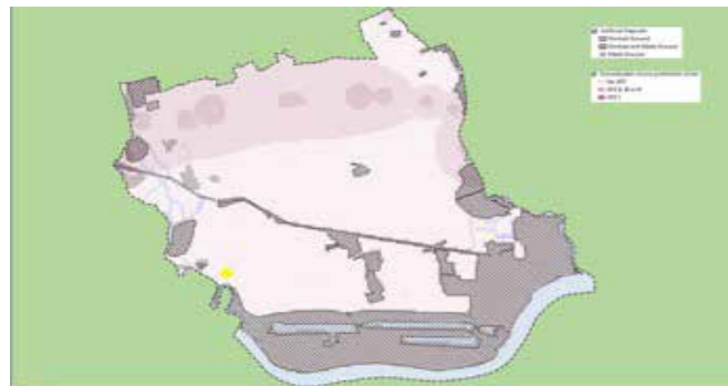
Fig.5 Newham's main made ground (grey/grey hatched) and source protection zones (shades of pink)
