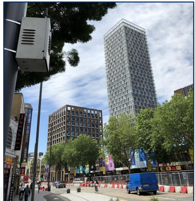
Lamp column particulate monitor, Stratford High Street
